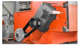
Less vibration with flexible set up with hard rubber feet
