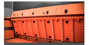
CONTROLLED MATERIAL FEEDING by ram with serrated plate and segmented floor
