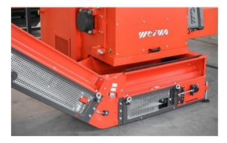
For most applications, electromechanical drives are the classic choice because they are easy to maintain and robust. WEIMA's special feature: we manufacture our own gearboxes that are specially designed for shredding operations. Torque monitoring and shockabsorbing vibration dampers round off the package. A hydrodynamic start-up clutch is available as an option for further protection of the machine. For even higher requirements, we recommend the use of a hydraulic drive.
