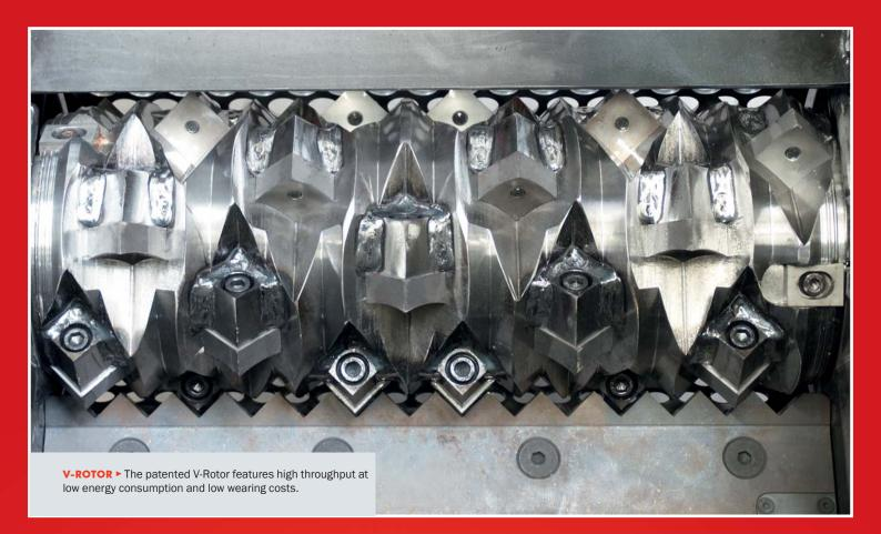
**FLEXIBLE AND POWERFUL.** The three available designs of the Spider HRS and the different rotors and knives allow for optimal reduction of materials such as plastic, paper, foil, filaments, wood or textiles.
